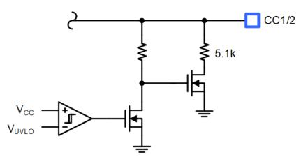
Figure 4. Simplified Schematic for Dead Battery Automatic 5.1kΩ Pull-Down Sub-Circuit
