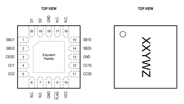
20-Pin 3mm x 3mm x 0.55mm UQFN Package, 0.4mm pitch Top Mark XX = Device ID Code, YW = Date Code, Z = Serial Number
