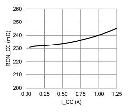
SBU Switch RON vs. Switch Current
