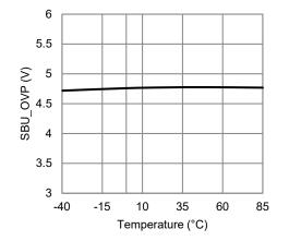
SBU Switch OVP Level vs. Temperature
