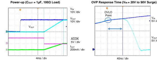
$V_{IN} = 20V$ ,  $C_{IN} = 0.1\mu$ F,  $C_{OUT} = 1\mu$ F, OVLO pin = GND,  $T_A = 25^{\circ}$ C unless otherwise specified.
