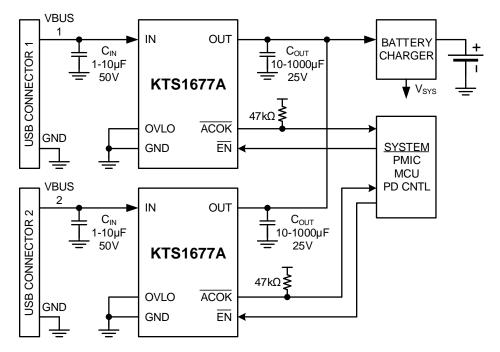
Figure 8. Two Input USB Adapter Configuration
