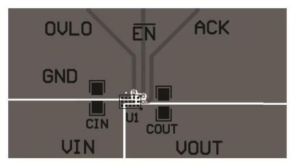
Figure 7. Recommended PCB Layout for WLCSP53-15 Package
