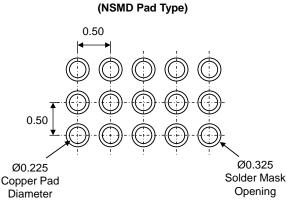
\* Dimensions are in millimeters.
