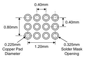
\* Dimensions are in millimeters.
