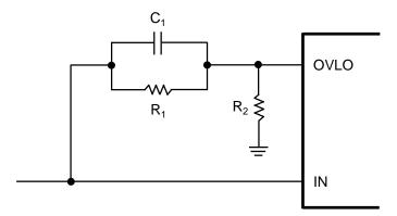
Figure 2. External OVLO Set Circuit
