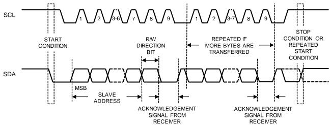
Figure 2. Data Transfer on I<sup>2</sup>C Serial Bus
