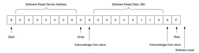
Figure 5. I<sup>2</sup>C Software Reset
