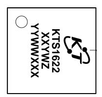
24-Lead 4.0mm x 4.0mm x 0.75mm TQFN44-24 Package
