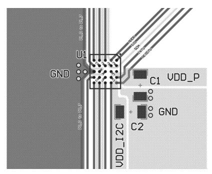
Figure 7. Recommended Layouts for FO-WLP55-25
