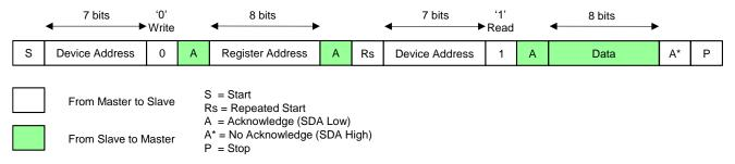
Figure 4. I<sup>2</sup>C Read Cycle
