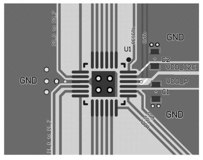
Figure 8. Recommended Layouts for TQFN44-24
