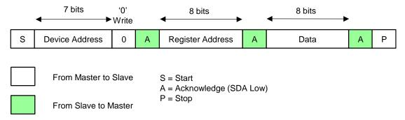
Figure 3. I<sup>2</sup>C Write Cycle
