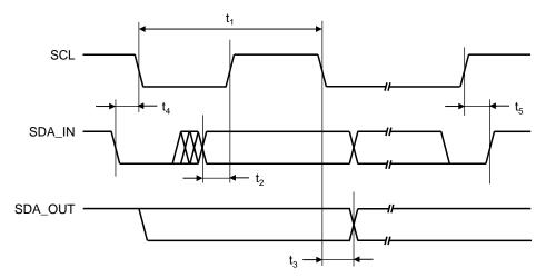
Figure 1. I<sup>2</sup>C Compatible Interface Timing
