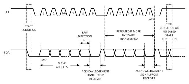
Figure 4. Data Transfer on I<sup>2</sup>C Serial Bus
