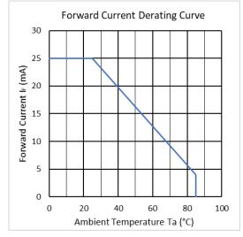
Figure 7. Forward Current Derating Curve
