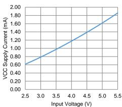
VCC Supply (No-Load) Current vs. Supply Voltage
