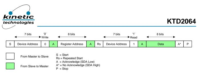
Figure 6. I<sup>2</sup>C Read Cycle
