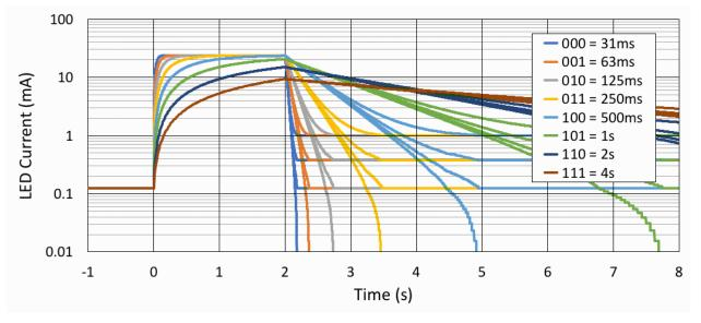
Figure 3. LED Brightness (current on log-scale) vs. Time vs. Fade Engine Time-Constant
