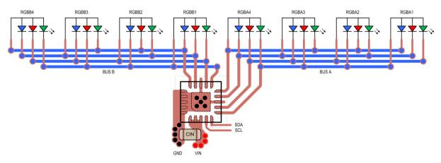
Figure 9. Recommended PCB Layout (light-bar example)
