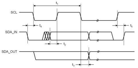
Figure 1. I<sup>2</sup>C Compatible Interface Timing
