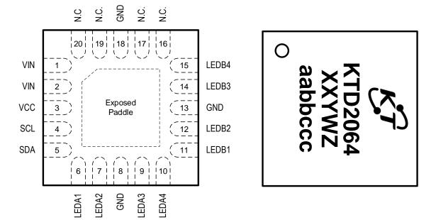
20-Pin 3mm x 3mm x 0.52mm UQFN Package, 0.4mm pitch Top Mark XX = Device ID Code, YW = Fab Date Code, Z = Serial Number aabbccc = Assembly Date Code
